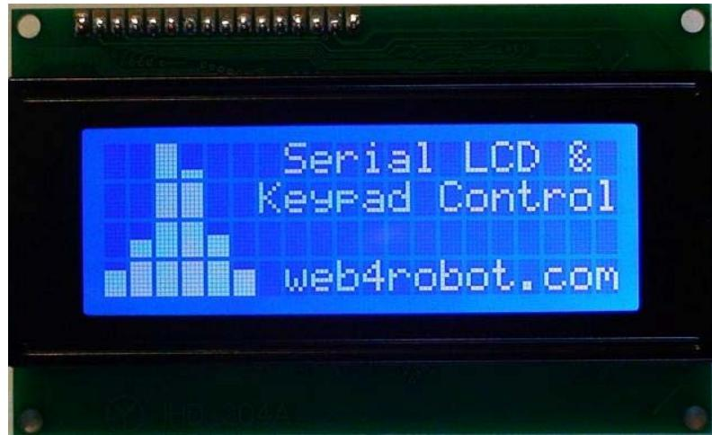
**LCD Module with I2C / Serial Interface and Keypad Control**
