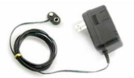
or it would be pretty easy to make your own from an old 9 to 12 volt wall transformer. Just remember that the buttons on the battery clip should be the reverse (male / female) of what they would be if clipped on a battery.
